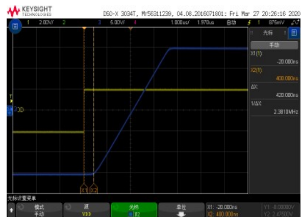
Time: 2 us/div, Measure Time: 420 ns R_L = 2\text{ k}\Omega , C_L = 100\text{ pF} , G = 10
